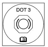
Your brake master cylinder reservoir is filled with DOT-3 brake fluid. See Engine Compartment Overview on page 373 for reservoir location and access.
